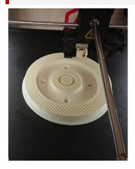
Mon-Chan has was able to create inner structure engineering using the rich parameters and comprehensive slicing preview provided by ideaMaker. By modifying structure features such as shell number, infill rate, infill structure, extrusion width, and layer height, Mon-Chan tried to redefine the mechanical properties of the workpiece against possible stress loading onto current geometry.
