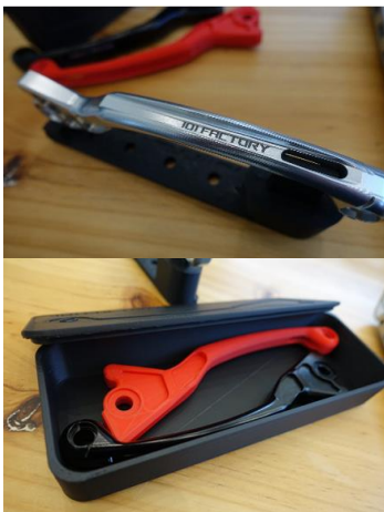
Jig (Up) for laser engraving within 3D printed packing (Down)
