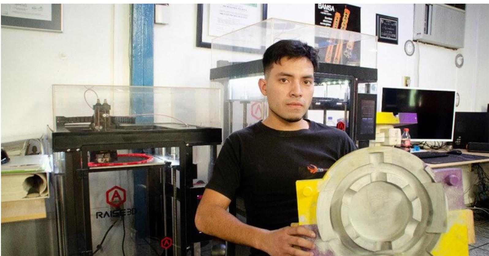
The molding process is formed by core making, mold making, and casting. The first phase is the most time-consuming, which is a challenge for the design and assembling process, requiring hand-making skills. 3D printing provides a shortcut to create the core with less time, less labor, less cost, and higher precision.
