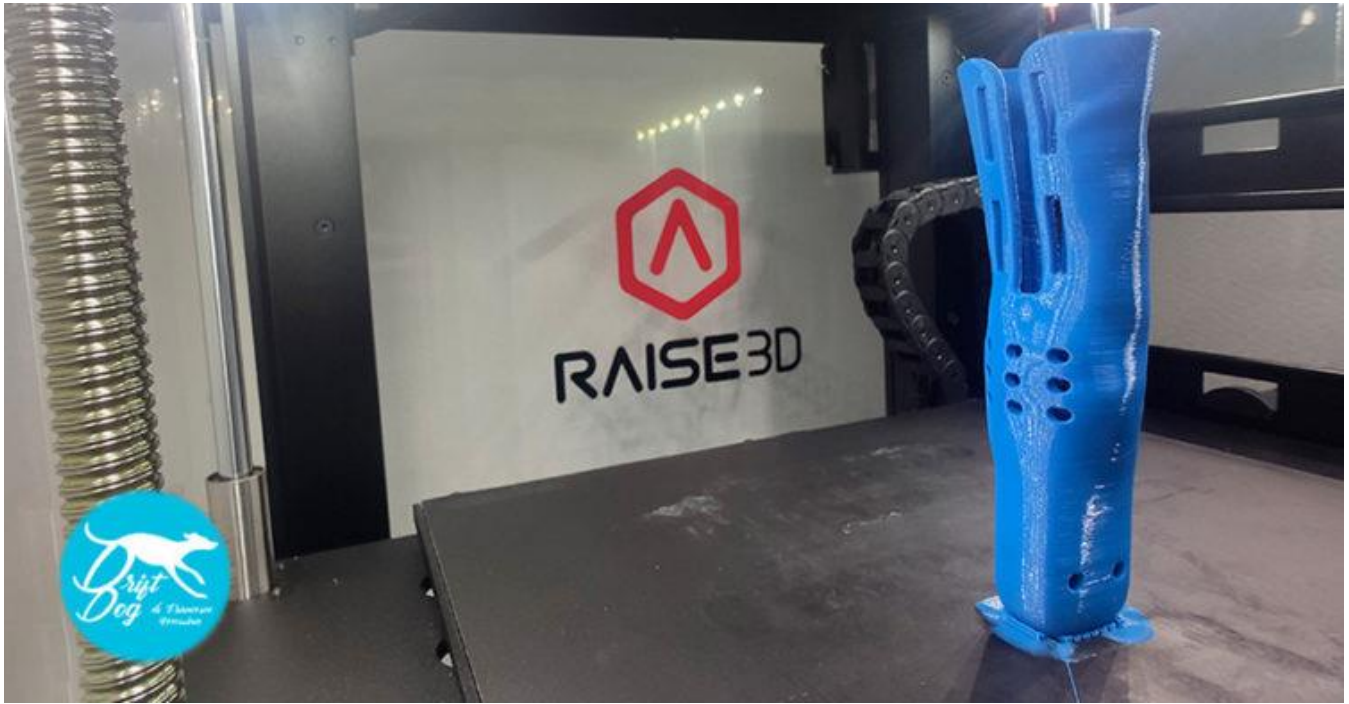
3D-printed prosthetic component made of TPU
