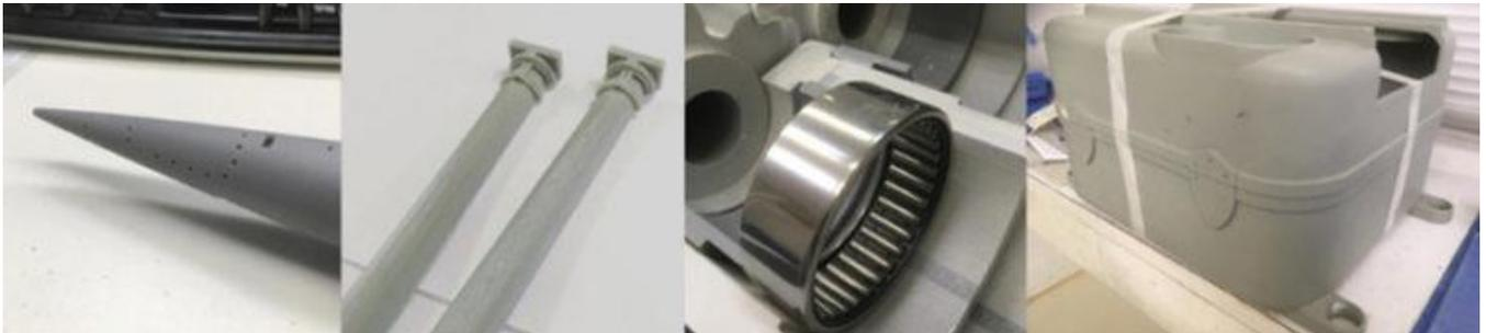
First, the Pro2 can print at small layer heights for a smoother surface on the final 3D printed object. Wamokei uses a 0.01mm layer height to deliver a smooth surface with minimal post-processing, such as putty or polishing.
