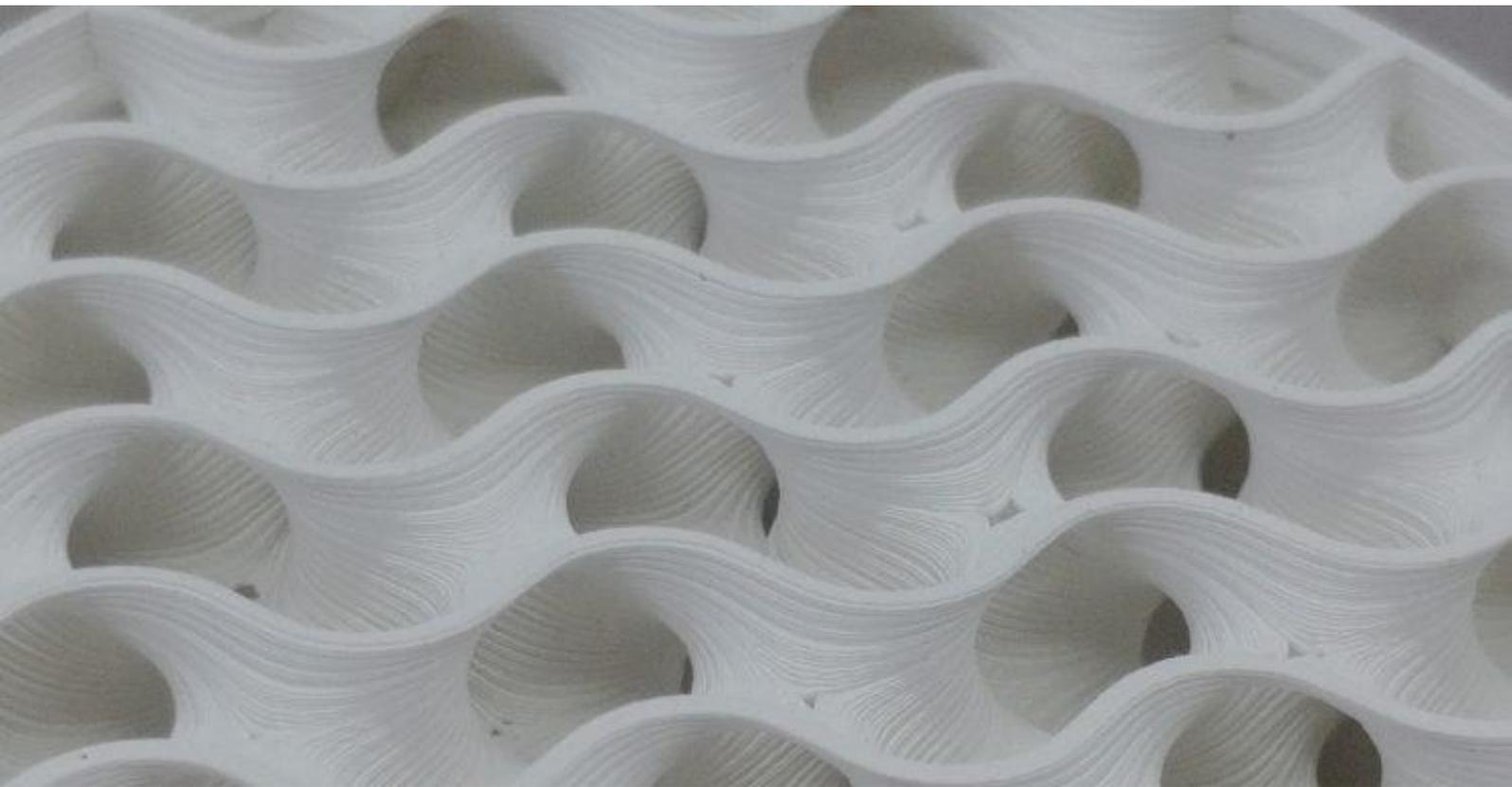
Avignon Ceramic produces ceramic parts for foundry, aerospace, and energy industries. The company is historically an expert in ceramic injection molding and produces cutting edge parts such as aerospace cores. **For 3 years, Avignon Ceramic prints its own parts thanks to ceramic additive manufacturing.**
