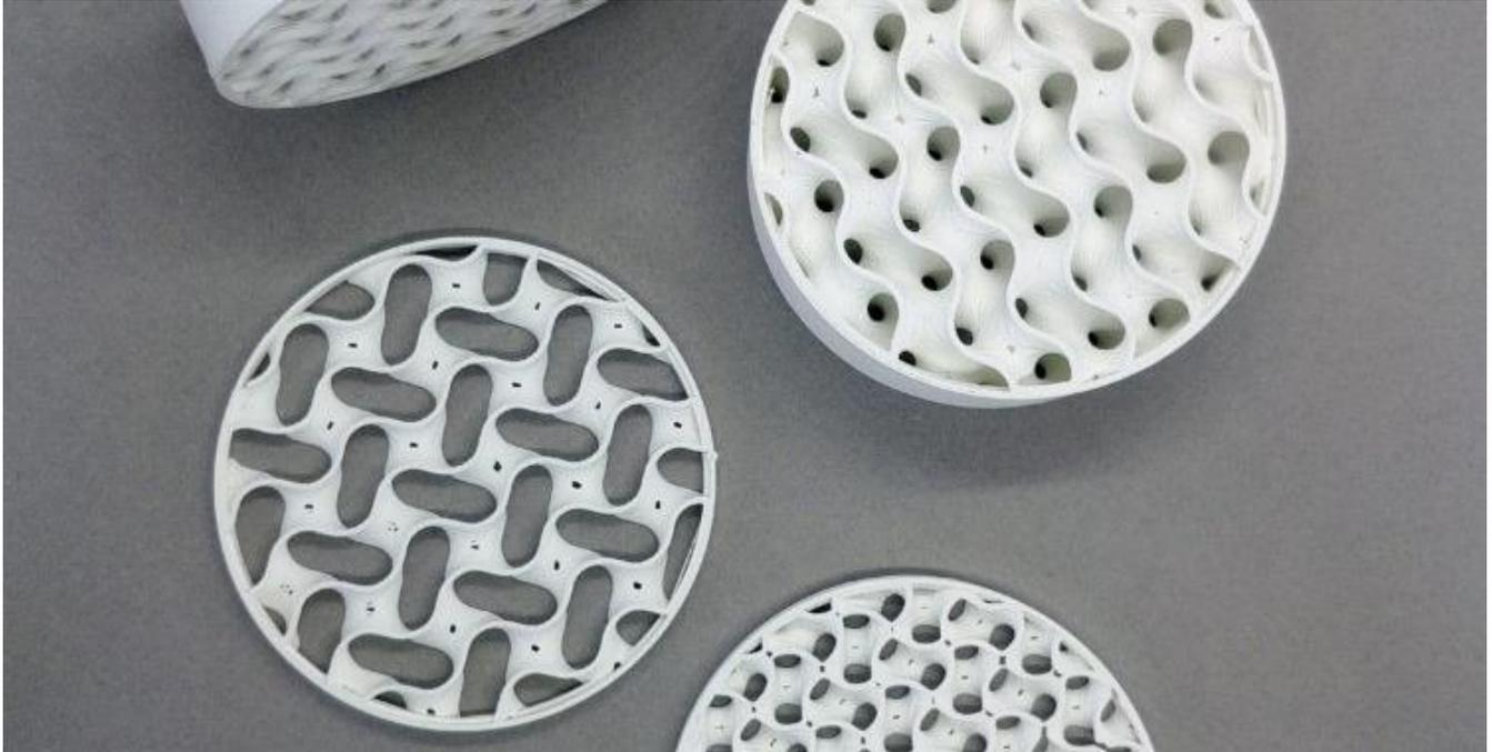
In the field of foundry, ceramics is an excellent choice to produce consumable tools, including ceramic filters. Ceramics is the only material that is high temperature resistant and chemically stable.
