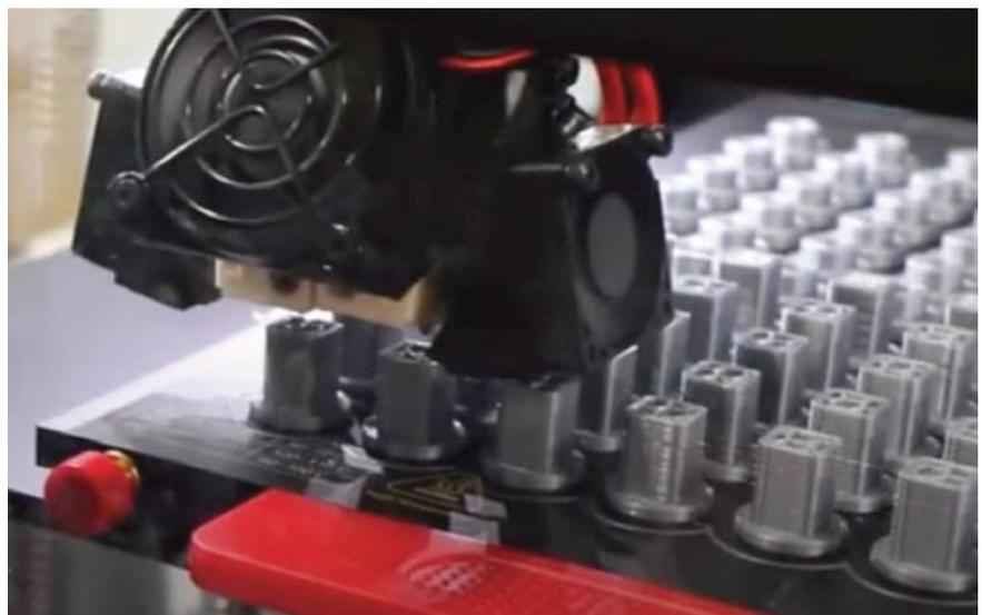
Printing Batch of Plastic Fixtures with the [Raise3D Pro2 Printer](#)
