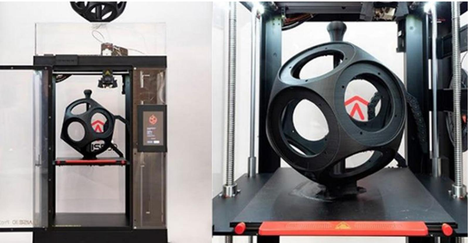
Recently NTEK revolutionized the production process of their Omni 4" Series focusing on 3D printing. With their trusted 3D technological partner Crea3D, NTEK designed and developed the new dodecahedral (structure with 12 sides) speakers, which radiate sound uniformly in all directions. The 360° surround sound facilitates accurate insulation measurement and reverberation time both in building and architectural acoustics.
