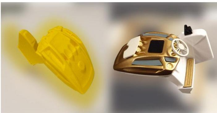
After creating a CAD file using a 3D design software, he uploaded the file to Raise 3D's patented slicing software ideaMaker to establish the print settings and determine how to assemble all the various pieces. Then, he created all the individual pieces of the hull and structure out of PLA. The swappable dual extruders support dual color prints (as shown) as well as an unmatched resolution that translates to a beautiful, smooth finish on the
