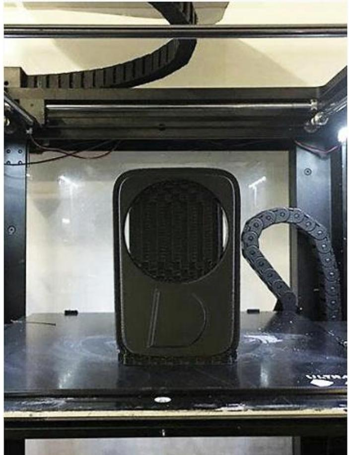
When manufacturing any type of replacement part or add-on to an existing vehicle; fit, tolerances, and precision are all major elements that need to play along with the visual elements desired in an automotive interior. **By integrating [Raise3D](#) additive manufacturing, DRAKES has elevated its manufacturing process to directly print final pieces in a faster and more accurate process than traditional fabrication.**
