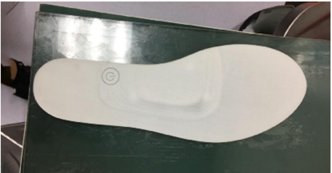
Insole printing exposed circuit slot on Raise3D N2.
